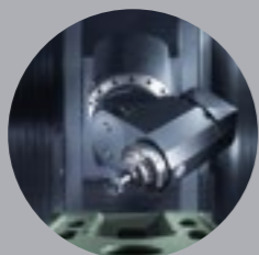
THC_B axis head Maintain the same tool center point across the full range -15^{\circ}/+195^{\circ}
